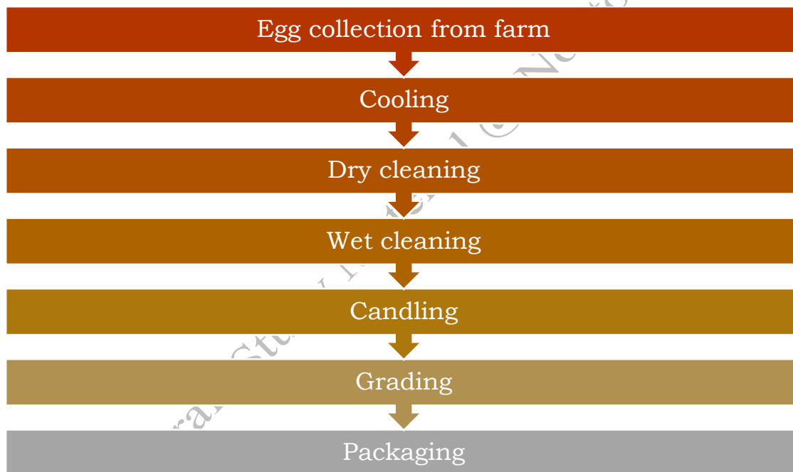
Fig.1.6: Steps of egg processing
