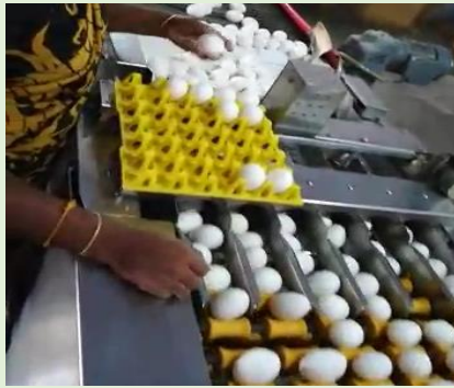
Fig.1.14: Sorting of eggs for shape abnormality
